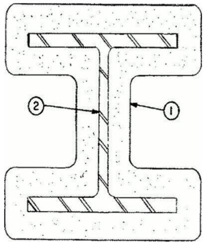
1. **Spray-Applied Fire Resistive Materials\*** — See table below for appropriate thickness. Applied in several coats to steel surfaces which must be clean and free of dirt, loose scale and oil. Min avg density of 35 pcf with min ind density of 32 pcf. For method of density determination, refer to Design Information Section, Sprayed Material. This SFRM has not been evaluated for patching.
